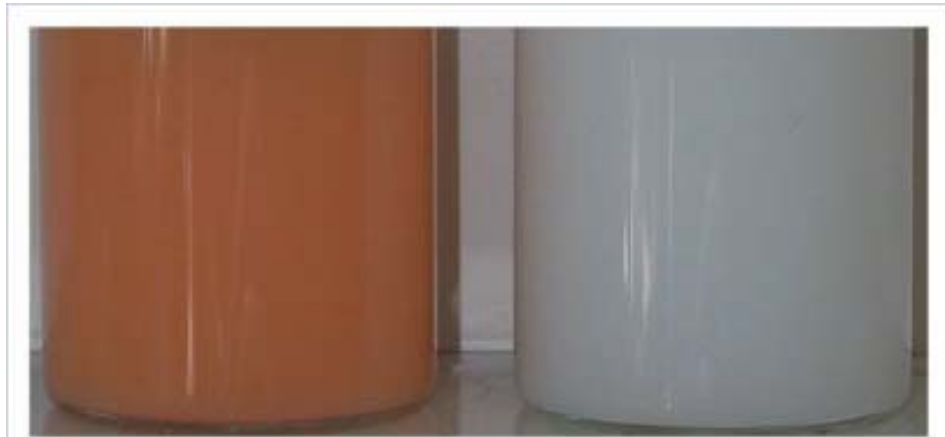
Photograph of the neat 100 nm latex (right) particles and the particles after dyeing by sorption with the hydrophobic pigment Sudan IV (left).
